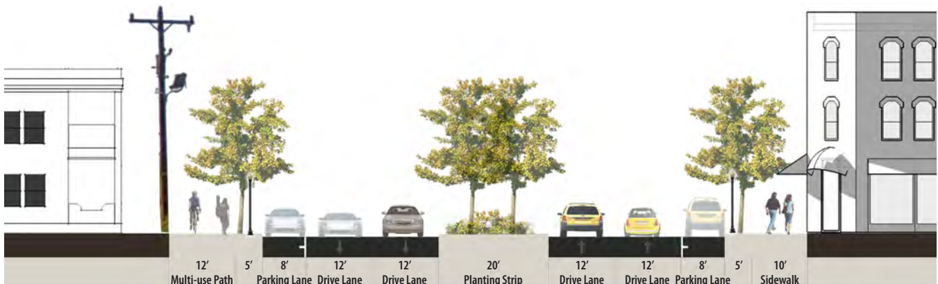
Pete Hollis Boulevard - Proposed Long-term Design Changes: Permanently reclaim outside travel lanes for parking at 8 feet in width. Narrow remaining four travel lanes to 11 feet in width. Expand center spot medians to 20 feet with reclaimed width and formalize as channelized medians with two rows of trees to create a parkway aesthetic. Create wider sidewalks in conjunction with new development.
