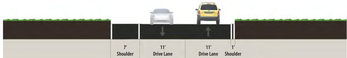
East Bramlett Road Bridge Segment - Proposed Design Changes (Option 1): Reduce vehicle lane size on the bridge segment (over the railroad adjacent to the Swamp Rabbit Trail) from 12 feet to 11 feet to allow a wider shoulder on the south side for pedestrians and cyclists, which would connect to the new sidewalk.
