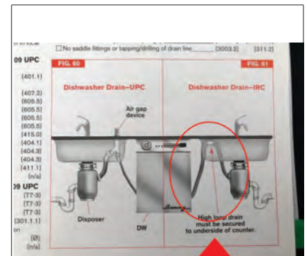
See above diagram for dishwasher drain to be highlooped
