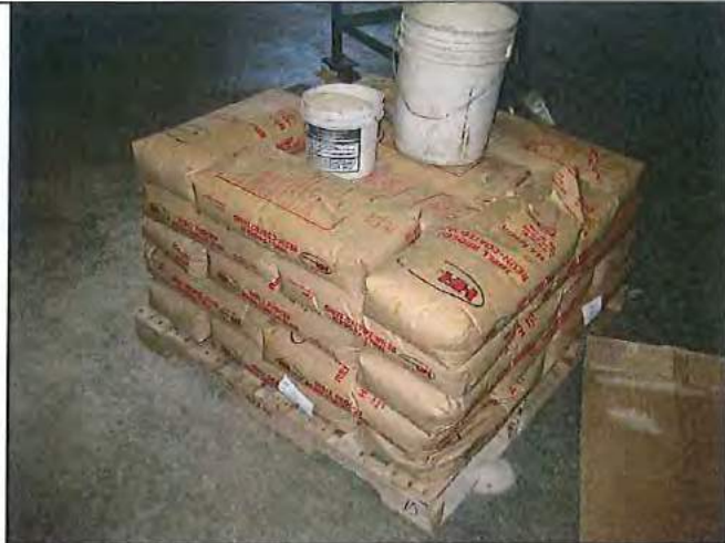
3. Pallet of unused resin coated sand (i.e., precursor of waste material)
