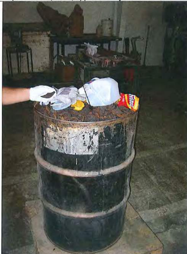
1. Drum with waste sand core molds. Arrow indicates approximate site of S-1.
