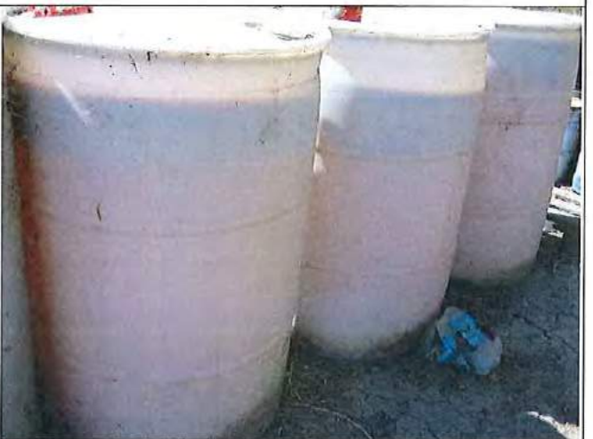
8. Close up of 3 westernmost drums in frame 7. Note apparent color differential of contents, indicating possible comingling of wastes
