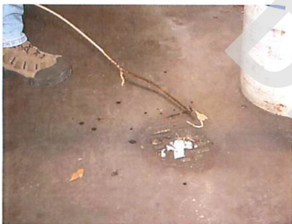
Photo ID # IMG_768/10:45 AM – Oil on dipstick used to test floor drains. This drain is adjacent to the oil storage room.
