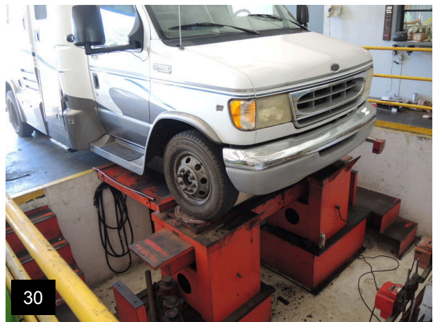
30 Recessed flooring for car alignment
