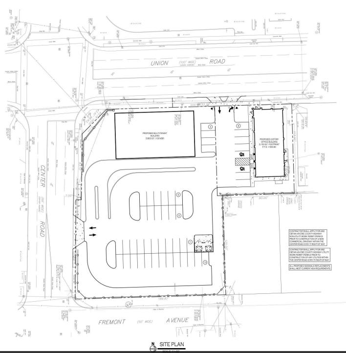
Concept site plan for a QSR tenant with a two-lane drive-thru
