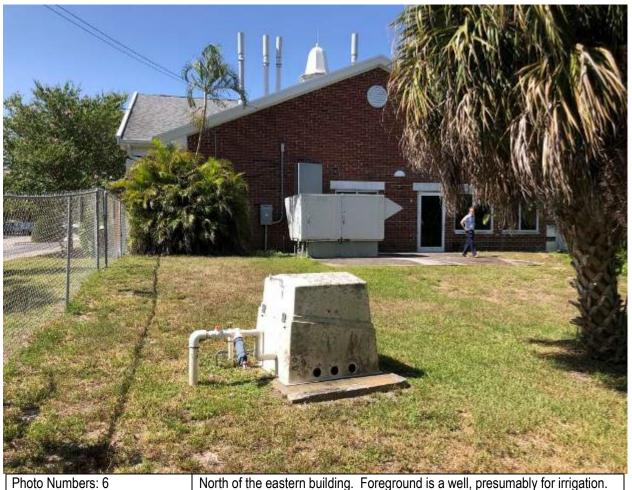
Photo date: 7/15/2022 Direction: S North of the eastern building. Foreground is a well, presumably for irrigation. Several vent pipes are evident in the roof of the eastern building – these are apparently for the exhaust hoods in the laboratory rooms.
