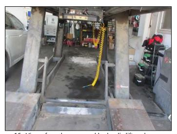
16. View of an aboveground hydraulic lift and new battery storage in the tenant space.
