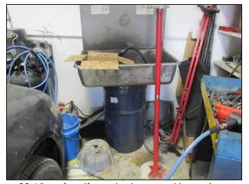
36. View of a self-contained parts washing station within the northern automotive repair tenant space.
