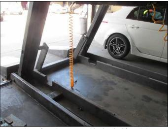
15. View of an aboveground hydraulic lift and *de minimis* oily staining on the concrete foundation
