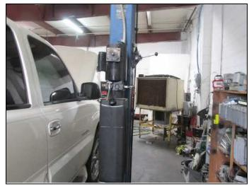
28. View of an aboveground hydraulic lift in the transmission repair tenant space.
